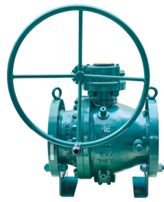
CS & FS TRUNNION BALL VALVE WCB & A105 | 6"-16" GO | 150# - 2500#
